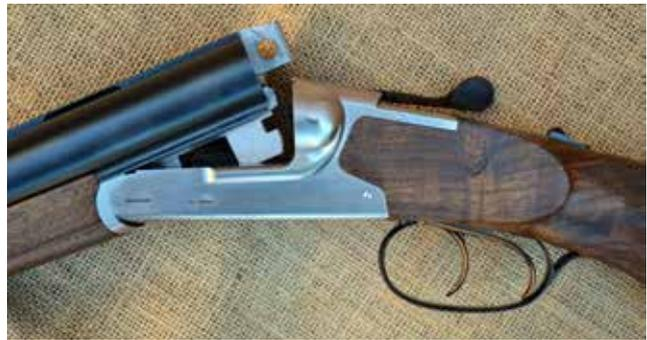
**A close-up of the Heym 88B action. Note the Greener cross-bolt, Purdey-style double underlugs, bolsters, double triggers and provision for telescope mounts in the rib.**
