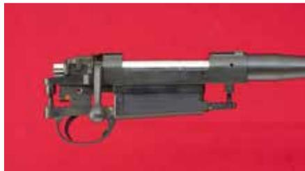
*The action has massive recoil lugs. The bottom of the action and the magazine are machined for the cartridge dimensions for each caliber to achieve perfect and reliable feeding. The magazine accepts four rounds for each caliber without using a drop box. As a result the rifle feels better.*
