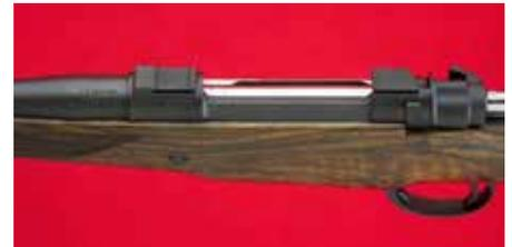
*The integral scope bases for Talley rings are low and include a front stop on both bases for additional security and safety. The fit of the metal to the wood is extraordinary. The fit requires care when removing the barreled action from the stock.*
